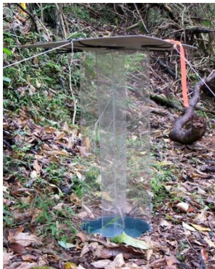
Figure 9.1: Flight intercept trap. Source: Deakin EL 2013. Impacts of land-use intensification on forest remnants embedded within production landscapes. PhD thesis, Canterbury University.
