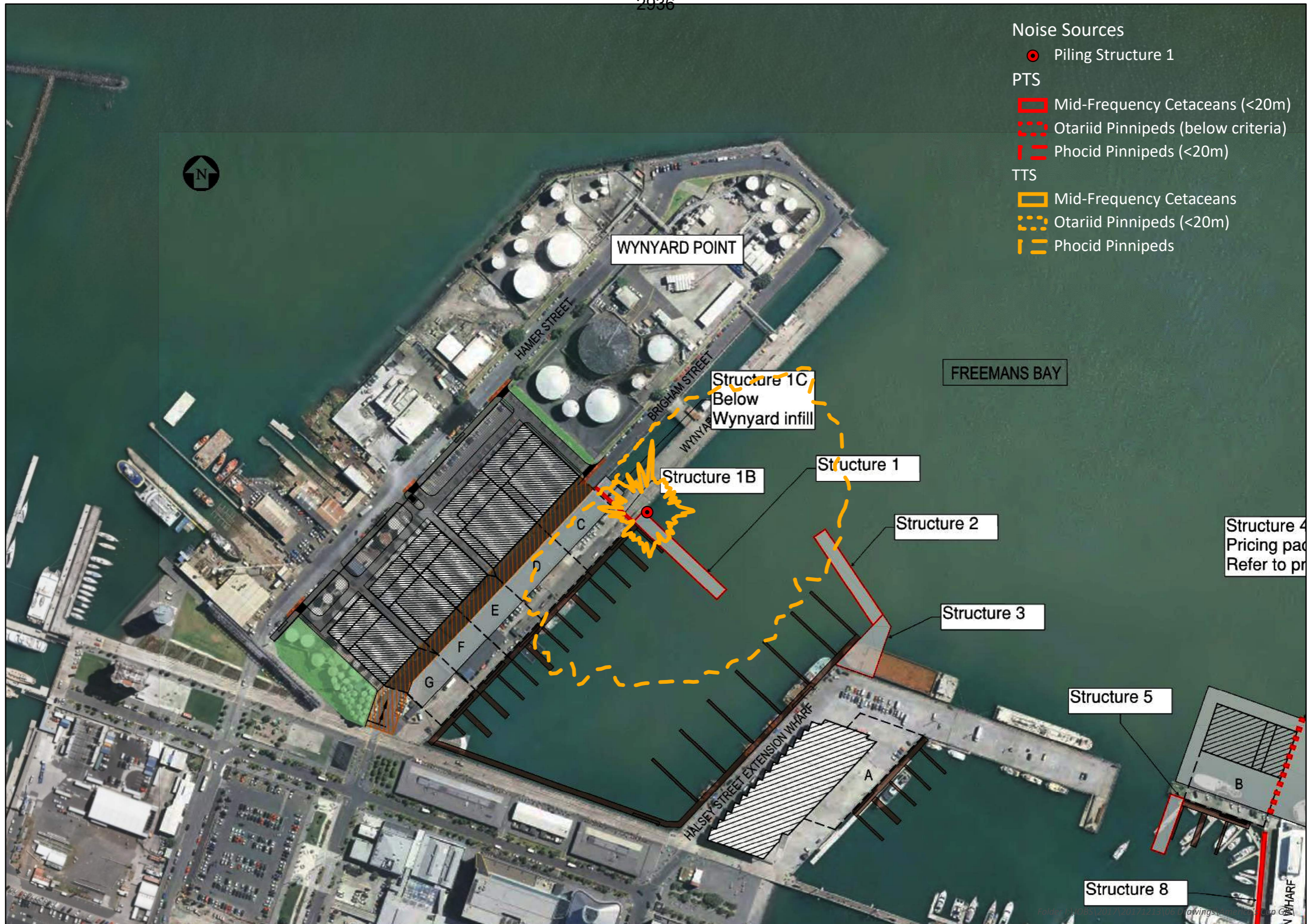
AC36 - Underwater Management Zones Figure 8: Structure 1 Impact Piling (1,200mm steel piles, 3 piles/day @ 50 strikes/pile)
