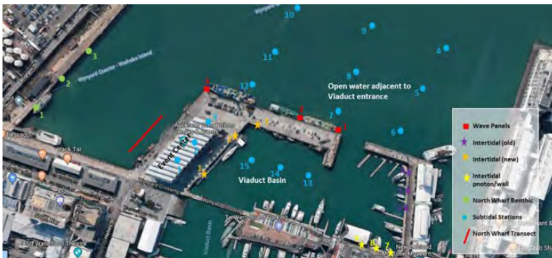
Figure 2-1: Sample locations for intertidal (wharf piles, pontoons, walls and wave panels), and subtidal surveys (sediment cores and video). Sediment stations were located under the Viaduct Event Centre on the Halsey Street Wharf Extension (Stations 1-3), in an area of open water in Freeman's Bay outside the entrance to the Viaduct Harbour (Stations 4-12), and in the Outer Viaduct Basin (Harbour) (Stations 13-15). An additional 30 m sediment transect was located in the corner of North Wharf and Wynyard Wharf. Intertidal Stations were located in the Outer Viaduct Basin (Harbour) on new wharf piles (Station 1-3), in the Viaduct Basin on old wharf piles (Stations 4-6), and in the Viaduct Basin on pontoons and walls (Stations 7-9). Wave panel sites were located on the external (open water side) of the Western Viaduct Wharf (Stations 1-3). Benthic habitat characterisation was located at the corner of North Wharf and Wynyard Wharf (Stations 1-3).
