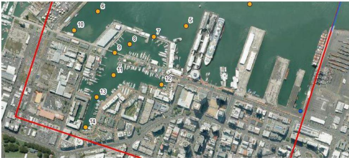
Figure 3: Tidal modelling output locations for the Wynyard Wharf South Waterspace and Viaduct Harbour (reproduced from Coastal Process Report, Figure 10).
