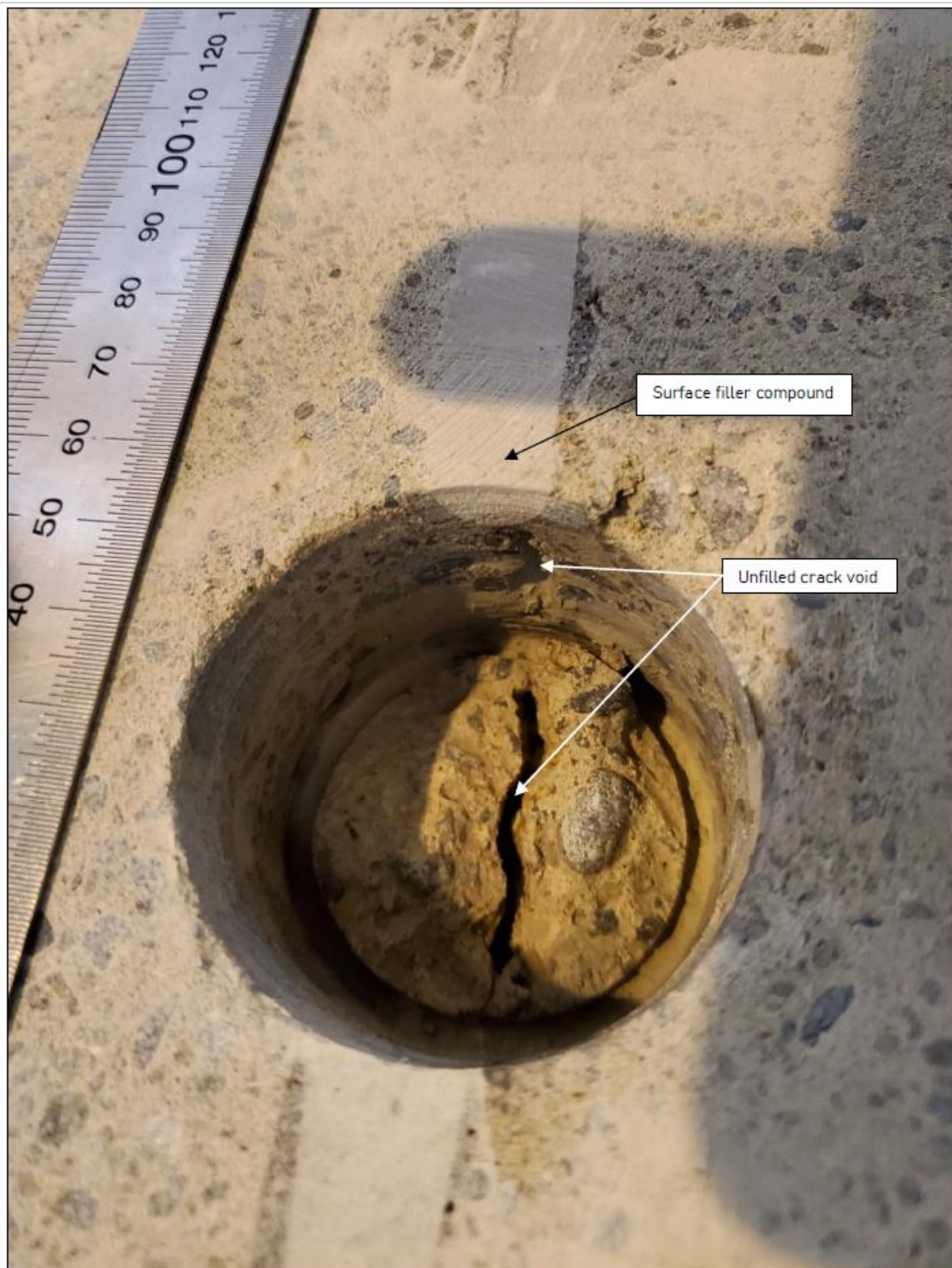
Photo 7: Close up view of cored hole. The penetration of the epoxy repair at this location is approximately 10 mm. There appears to be little in the way of structural epoxy filler material below the surface filler compound. This is a superficial surface repair.
