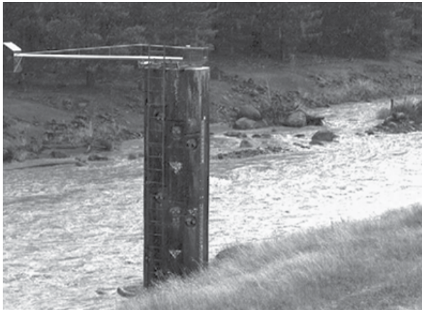
Lahar warning tower on the Whangaehu River, seen with the river at normal levels (left) and during a flood (right). The system was erected following the 1953 Tangiwai railway disaster and was designed to gauge the flow depth of water and send a warning 15 minutes before a lahar reached the railway bridge 11 kilometres down river.
